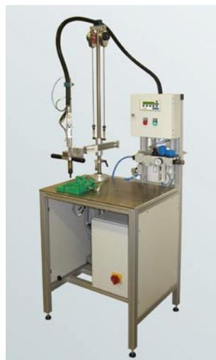
Speed Fastening® module with rivet process monitoring and release function at balancer arm for assembly of AC converter.
