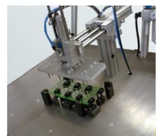
Multiple head workstations especially designed for assembly of various electronic components.
