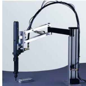
Single-head workstations provide rapid assembly which makes them cost-effective even with small batch sizes. Available as Pantograph, Fixed arm or Under-bench Workstation.
