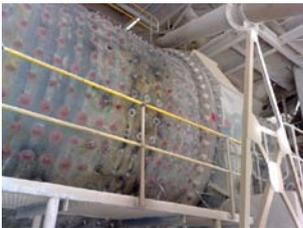
Cement mills - liner plates attached to the drum
