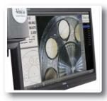
'Next generation' measurement software coupled with a high resolution video camera enables Falcon to measure a wide variety of simple and complex features, quickly and simply. Essential measurement data, with graphics-based "part view" construction is displayed alongside the high resolution video image.
